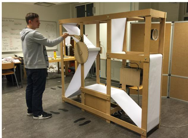
**Figure 1. The machine work in an assembly line manner so all the “stations” has to be operated at a time: Turning the handle enables the microphone -> talking into the microphone enables the lamp over the drawing station -> drawing on the paper enables a kinect and the beamer and finally interaction with with kinect will enable drawing with the beamer.**
